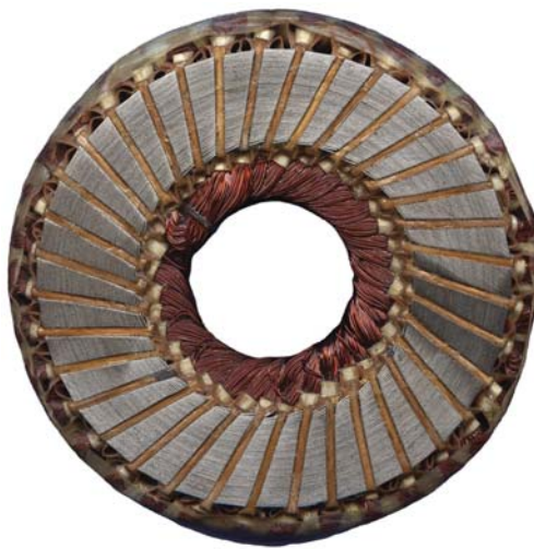
Genuteter Stator eines DSM-Motors Slotted stator of a DSM motor
