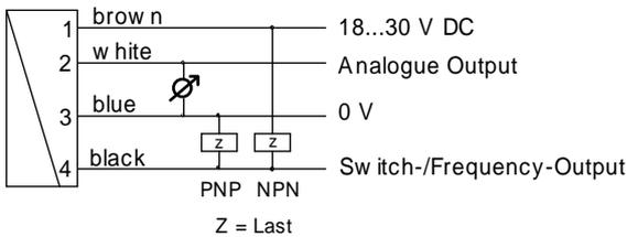
Please use shielded cable, signal lines < 30m and power supply lines < 10m.
