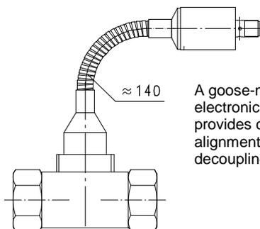
A goose-neck (optional) between the electronics head and the primary sensor provides complete freedom in the sensor alignment. This option also gives thermal decoupling between both units.
