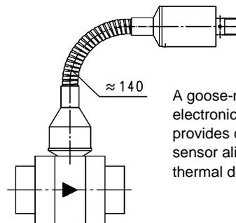
A gooseneck (optional) between the electronics head and the primary sensor provides complete freedom in the sensor alignment. This option also gives thermal decoupling between both units.
