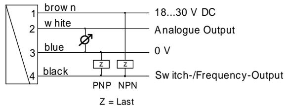
Please you use shielded cable, signal lines < 30m and power supply lines < 10m.
